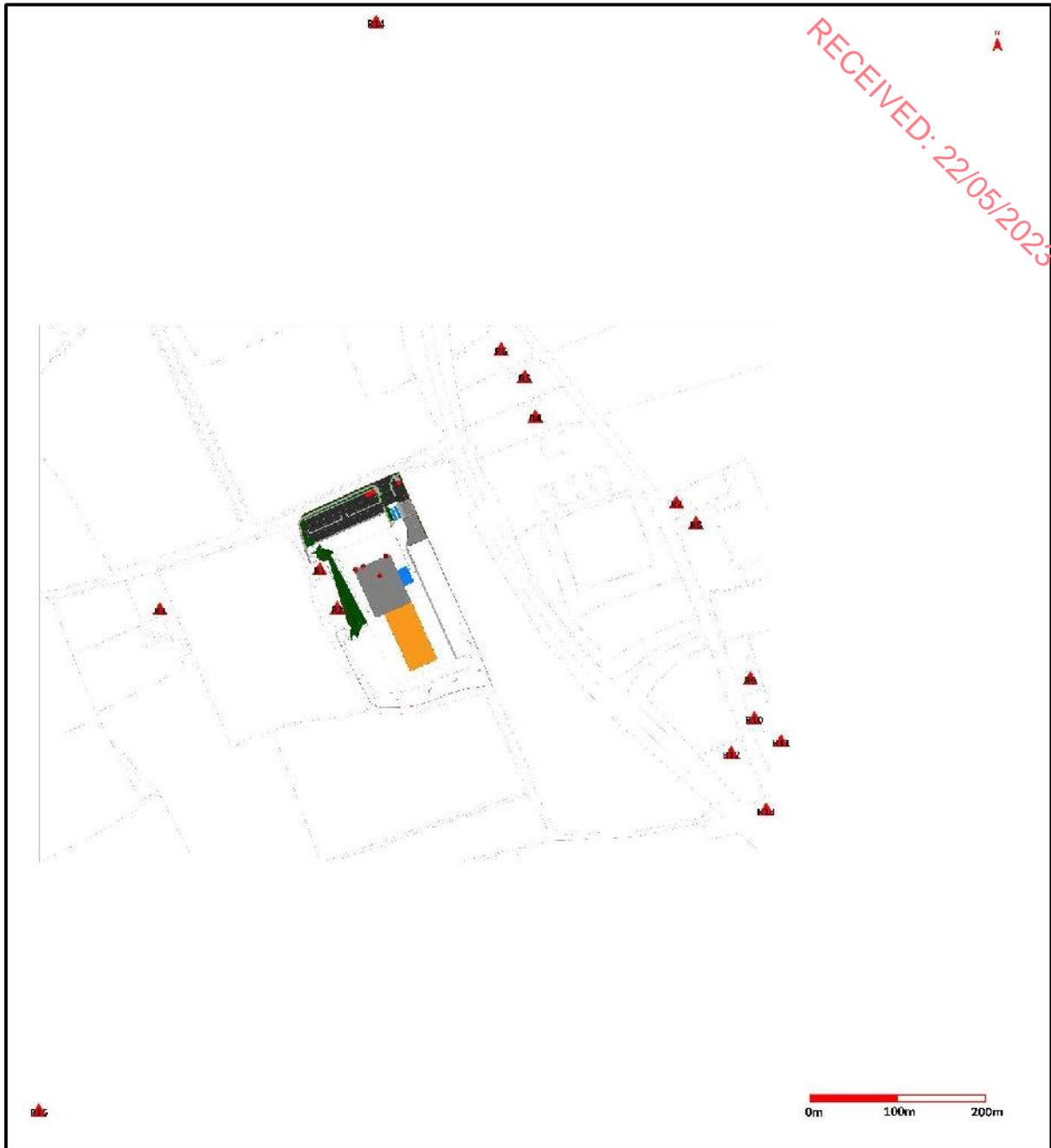
Figure 11.3. Hibernia Steel Facility layout, relative location of receptors and location of proposed emission points located within the boundary of the facility.
